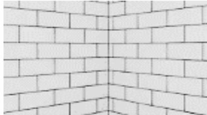
**BUTT JOINT CORNER** - Butt two panels together at the inside corner. If there are any unwanted gaps, the Stone Finish caulking can be used.
